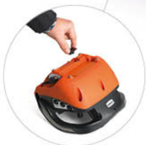
External removable EEPROM SIM module
