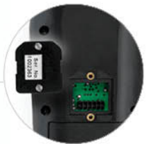
External removable EEPROM SIM module
