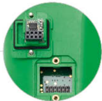
External removable EEPROM SIM module
