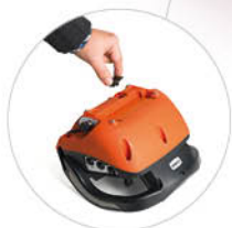
External removable EEPROM SIM module
