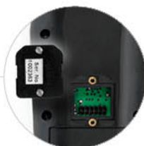
External removable EEPROM SIM module
