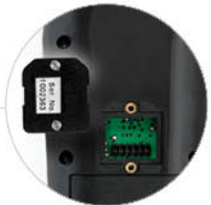
External removable EEPROM SIM module
