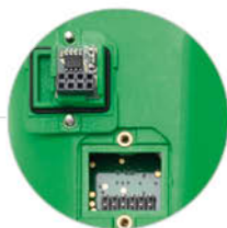
External removable EEPROM SIM module
